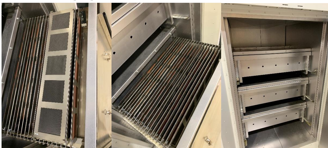
Picture 1-3. Example of sample specimen rack holder and the heat chamber equipment for 70 °C with air-speed of 5 m/s.
